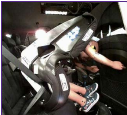
An example of belt routing misuse
