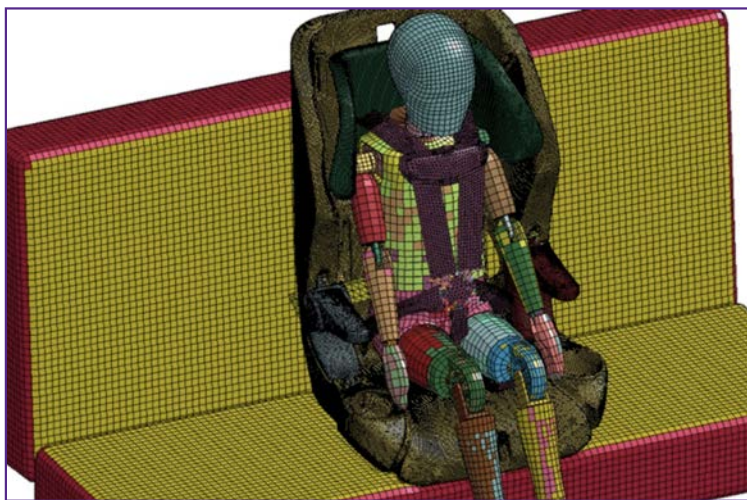
Hybrid III 6-year-old ATD in a forward-facing child restraint on the C/FMVSS 213 bench in a finite element simulation
