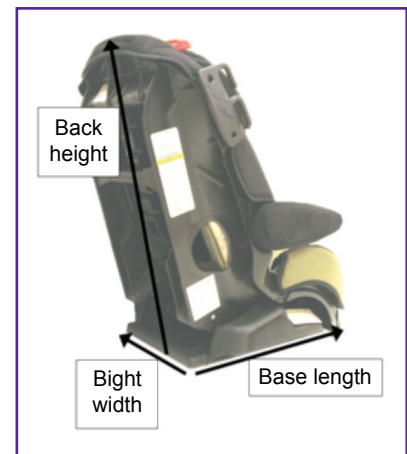
Several of the dimensions measured on each CRS are shown above.
