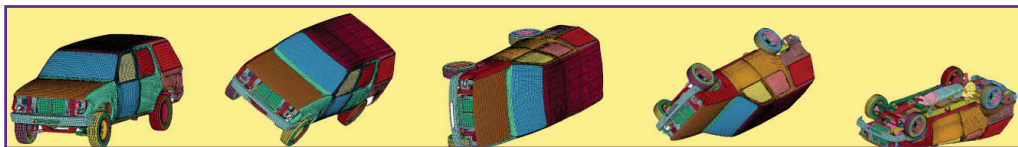
This finite element model depicts a rollover with two quarter turns.
