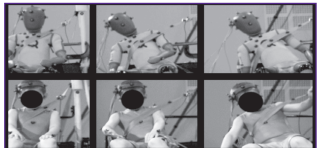
This image shows the kinematic comparison of the Q6s ATD (top) and exemplar 6-year-old volunteer (bottom) at initial position, mid-motion, and maximum excursion in a lateral low-speed impact. At mid-motion, the Q6s exhibited lateral head rotation, whereas the volunteer's head remained upright.
