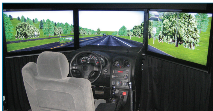
The driving simulator used as part of the Simulated Driving Assessment.
