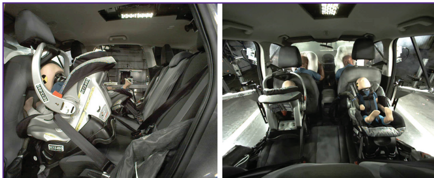
Freeze frame views of a rear-facing CRS installed in a forward-facing direction.
