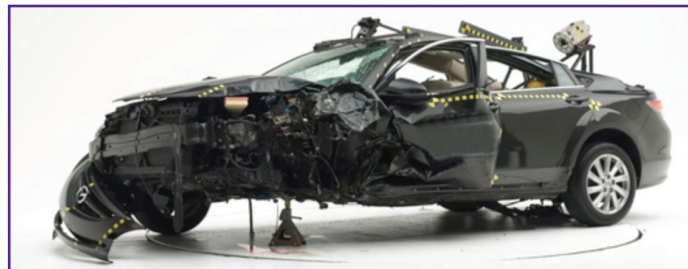
A post-test photo from the full vehicle small overlap crash testing (photo courtesy of the Insurance Institute for Highway Safety).
