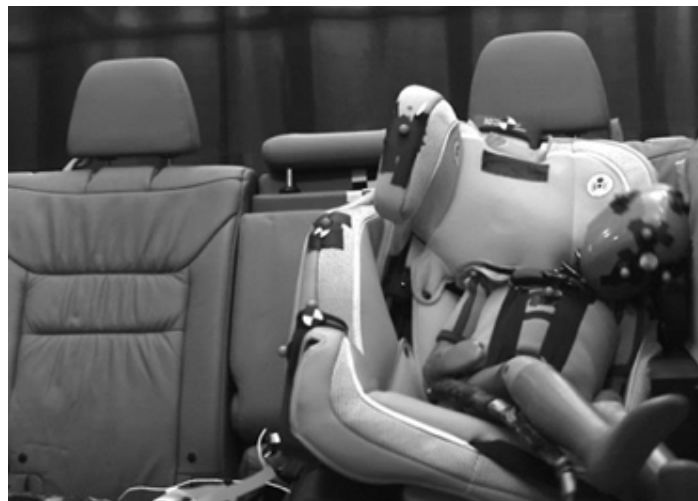
High-speed video frame at maximum head excursion, for the FF CRS tested in the untethered condition. Note CRS yawing and tipping and ATD lateral excursion and head impact with the simulated intruded door.
