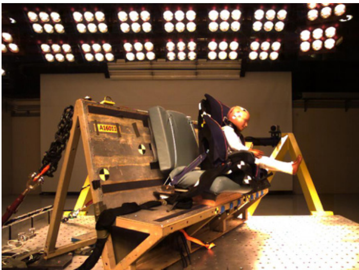
Sled test of a forward-facing CRS installed using a deactivated inflatable seat belt and Hybrid III 3-year-old ATD.
