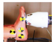
At left: The set-up for the repeatability tests is pictured. At right: The ram impactor making contact with the ATD-LE.
