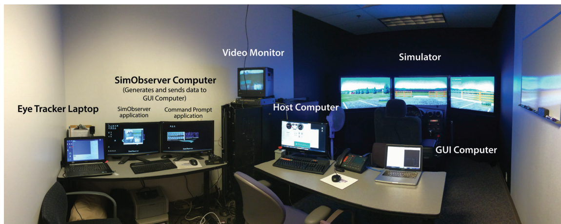
The simulator lab, housing a Pontiac G6 driver seat, LCD panels allowing for a 160 degree field of view, active pedals and steering system, and a rich audio environment.
