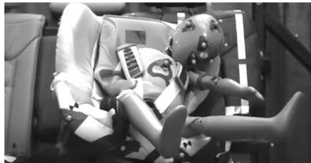
High speed video image of Q3s ATD kinematics at time of maximum excursion in rigid ISOFIX attached FF CRS without a tether. Inch tape line on right side of vehicle seat represents typical door or side structure intrusion.
