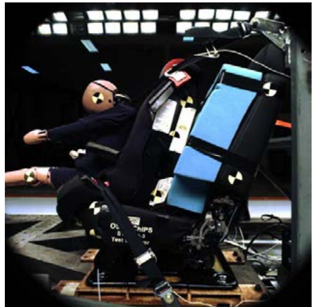
Booster seat occupant in a frontal impact, using a seat cushion shortened by the addition of the blue spacer.
