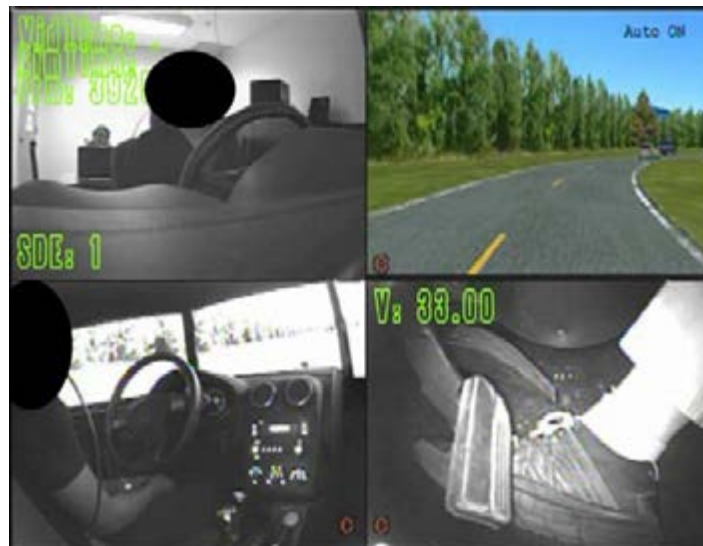
Top Left: Driver in the seat without hands on the wheel (View 1); Top Right: Two-Way scene; Bottom Left: Driver in the seat without hands on the wheel (View 2); Bottom Right: Foot under the pedal while in autonomous mode
