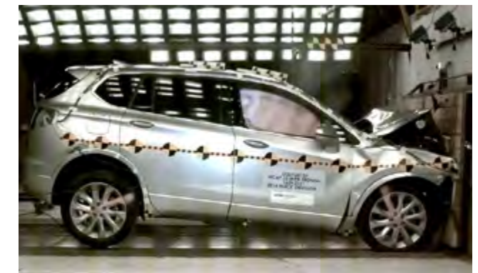
Frontal crash test showing pitching motion of the rear of the vehicle, which places vertical loading on the rear occupants.
