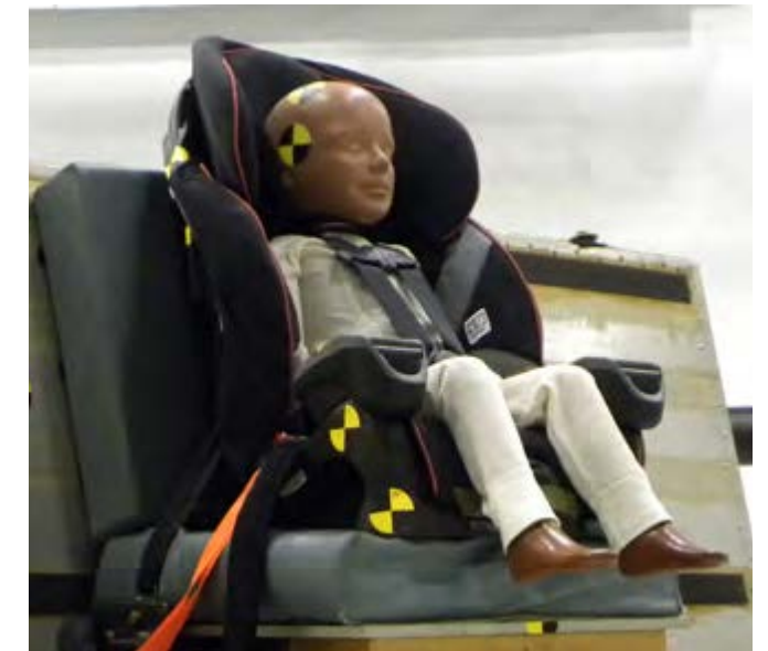
The 3-year-old Hybrid III ATD seated in a forward-facing CRS positioned for the 45 degree oblique test.
