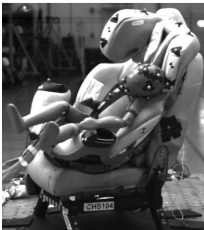
Image of a sled test showing the FF CRS rotating and tipping towards the impact direction, facilitating the ATD head to rotate around the FF CRS side wing.
