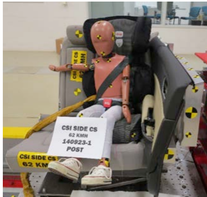
A Hybrid III 6-year-old ATD seated in a high-back booster seat restrained with a lap-and-shoulder belt is subjected to side-impact testing.
