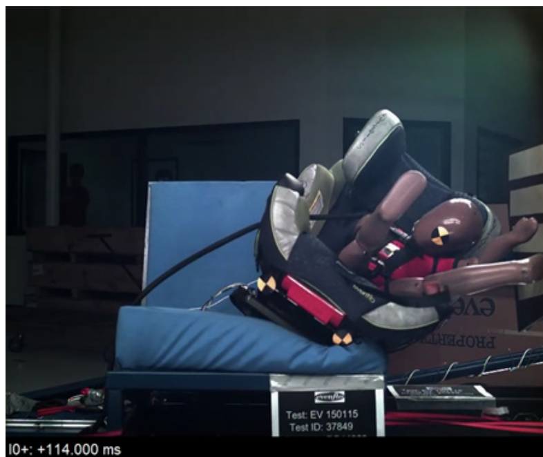
Video capture from a sled test of a far-side impact in which no top tether was used in the installation.
